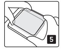
Align the glass straight down over lens.
